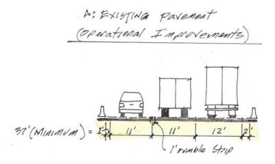
37' (minimum) – same as EB with 2 foot on right shoulder instead of 4. This could result in reduced speeds. Also reduces space for driver error. Some areas are wider (41' at some interchanges). Bridges are 38' wide. Shy on inside is 1' (same as EB).
