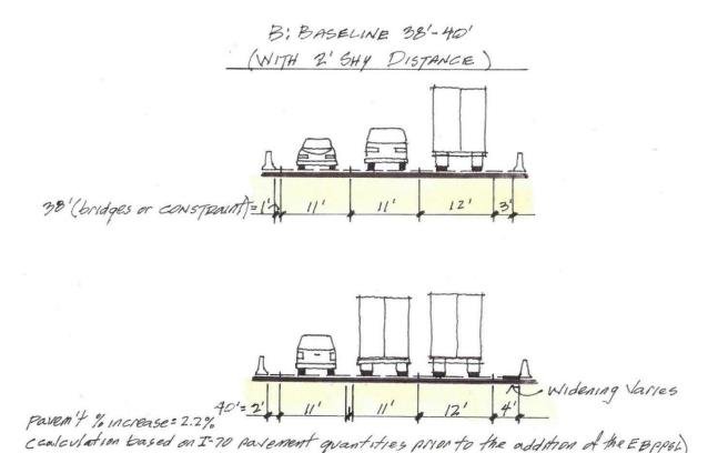
**CCC Comment:** The rumble strip is not a full foot, it is the width of the paint stripe. It is not taking 6 inches out of PPSL and adjacent GP lane. Putting a foot in for the rumble strip is superfluous because the strip is not 12 inches wide.
