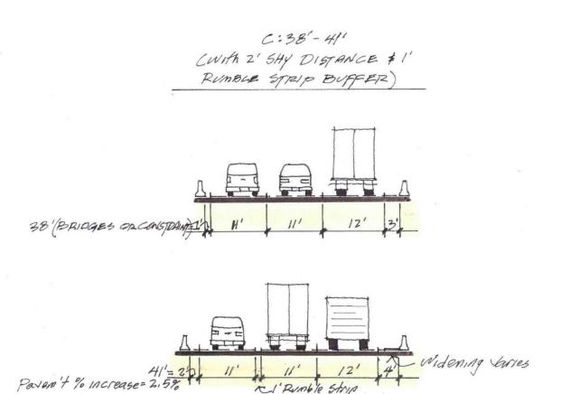
**CCC**: Can we just put the rumble strip outside the outside stripe like it is done in other locations? **A**: We need to place it between the lanes because if we placed it on the outside of the stripe it would encroach even more into an already narrow PPSL lane making the PPSL lane even more uncomfortable than it is already.
